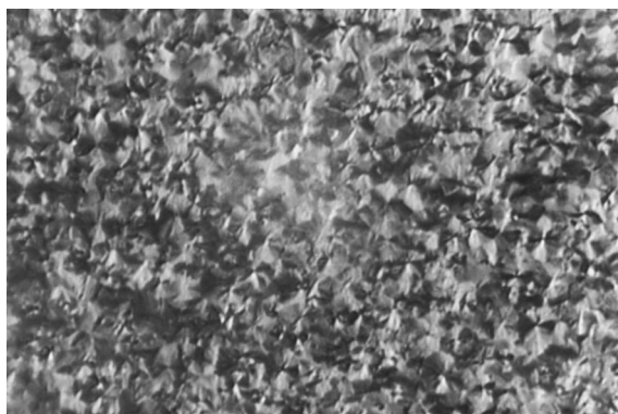
Fig. 3. The spherulitic structure of Terathane 2000 after crystallization at -20^{\circ}\text{C} ; 1 cm on the photograph corresponds to 19 mm in reality.
