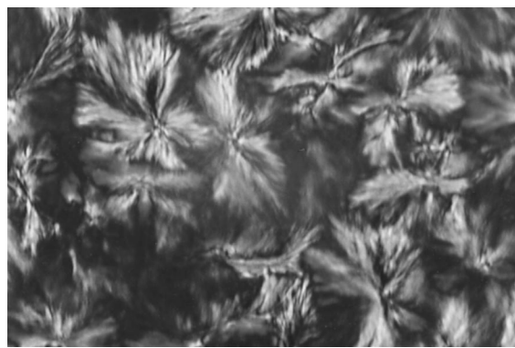
Fig. 4. The spherulitic structure of Terathane 2000 after crystallization at 18^{\circ}\text{C} ; 1 cm on the photograph corresponds to 19 mm in reality.
