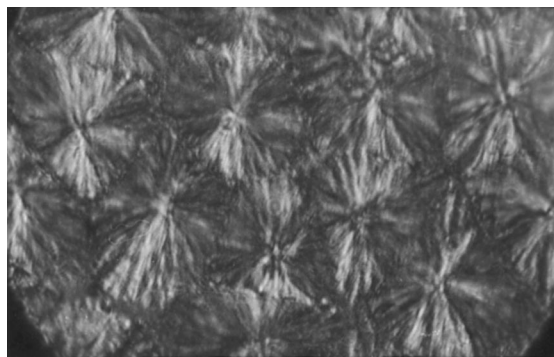
Fig. 6. The spherulitic structure of soft segments of the polymer obtained in a reaction of the prepolymer crystallized at 7°C (1 cm on the photograph corresponds to 5 mm in reality).
